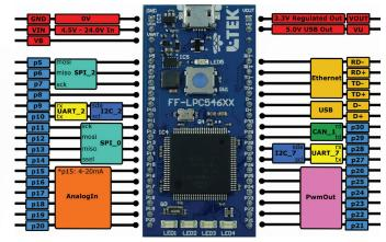
The pinout diagram above shows the commonly used interfaces and their locations. In addition to their stated functions, all GPIO pins can also be used as DigitalIn and DigitalOut interfaces.
