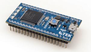
The L-Tek FF-LPC546xx is a small, 40-pin development board intended for prototyping general microcontroller applications. It is based on a low-power, peripheral-rich and debug capable NXP LPC54606 microcontroller enhanced with the powerefficient 220 MHz ARM<sup>®</sup> Cortex<sup>®</sup>-M4 core, with integrated DAPLink interface for a complete debugging experience.
