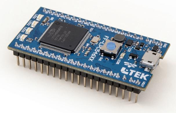
ARM® Cortex®-M4 USB Drag 'n' Drop Programming Online Compiler Mbed™ Enabled
